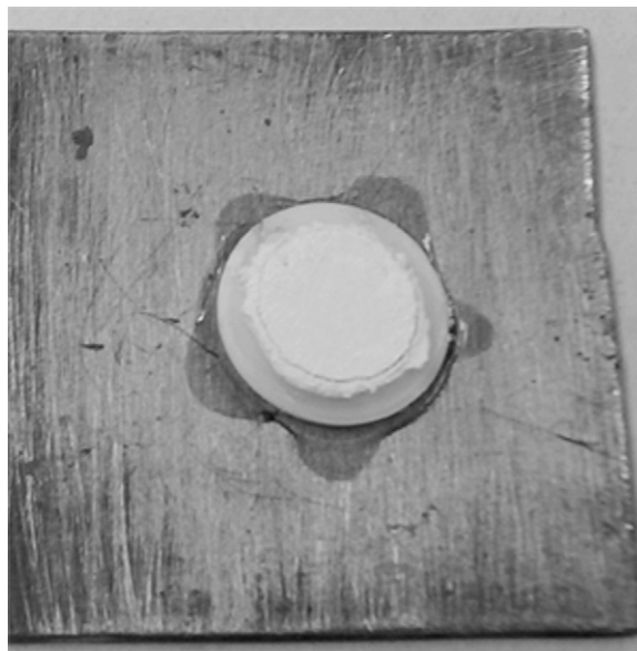
Fig. 3. Pasted electrode after curing. Internal volume of Teflon ® ring is 0.24 mL.
